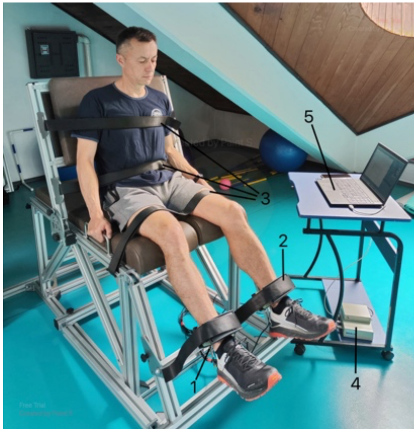
Picture 3. Testing setup. Subject in a custom-made chair (1: force transducer; 2: shanks; 3: rigid straps; 4: acquisition and analog-to-digital conversion unit; 5: monitor with visual feedback).
