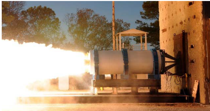
Figure 29 Solid propellant rocket motors L-block test stand [56]
