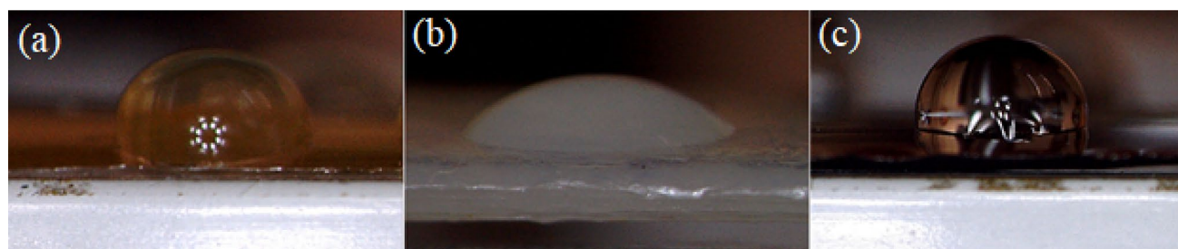
Fig. 3 Water contact angle for: (a) GAGP-PVP, (b) GAG-PVP-ALN and (c) GAG-PVP-GEN-ALN
