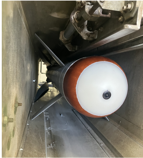
Figure 3.79: Fixed forward-looking nose camera used for real-time flight video transmission.
