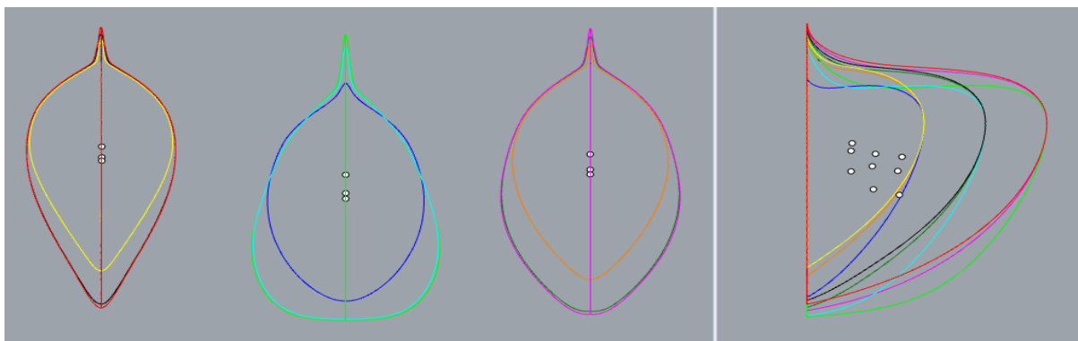
Fig. 3: \nabla -type, \Delta -type, O-type bulbous bows, respectively (transverse view (left) and longitudinal view (right))
