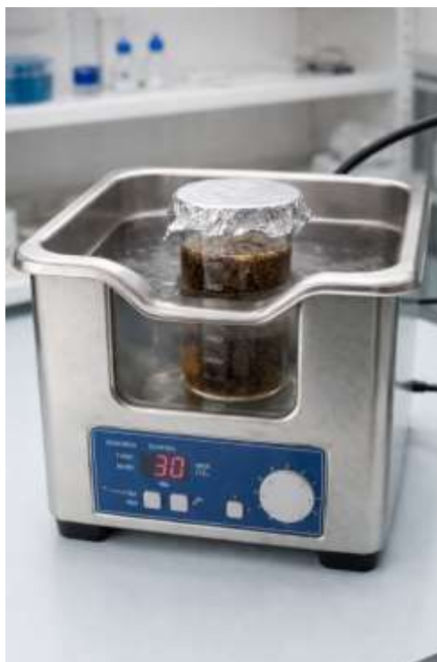
Figure 8. Ultrasound-assisted extraction of the smoke tree wooden part using ethanol in water (80%)
