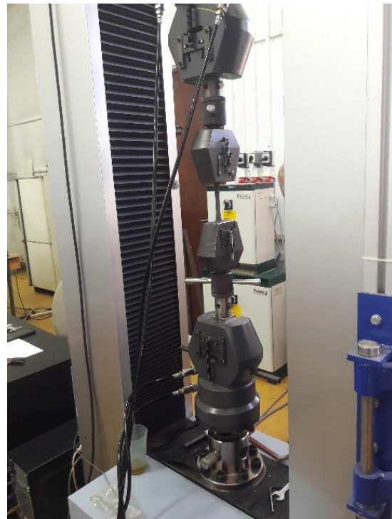
Figure 4.4 Experimental setup used for the tensile test
