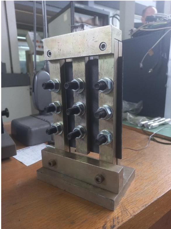
Figure 4.12 Specimen for shear testing inserted into Three-Rail Shear fixture
