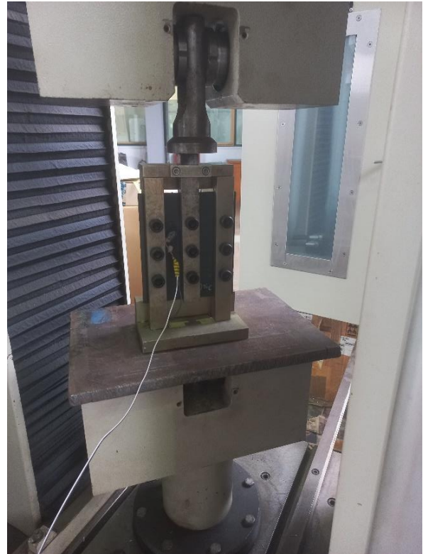
Figure 4.13 Three-Rail Shear fixture with specimen inserted positioned within the Universal Testing Machine
