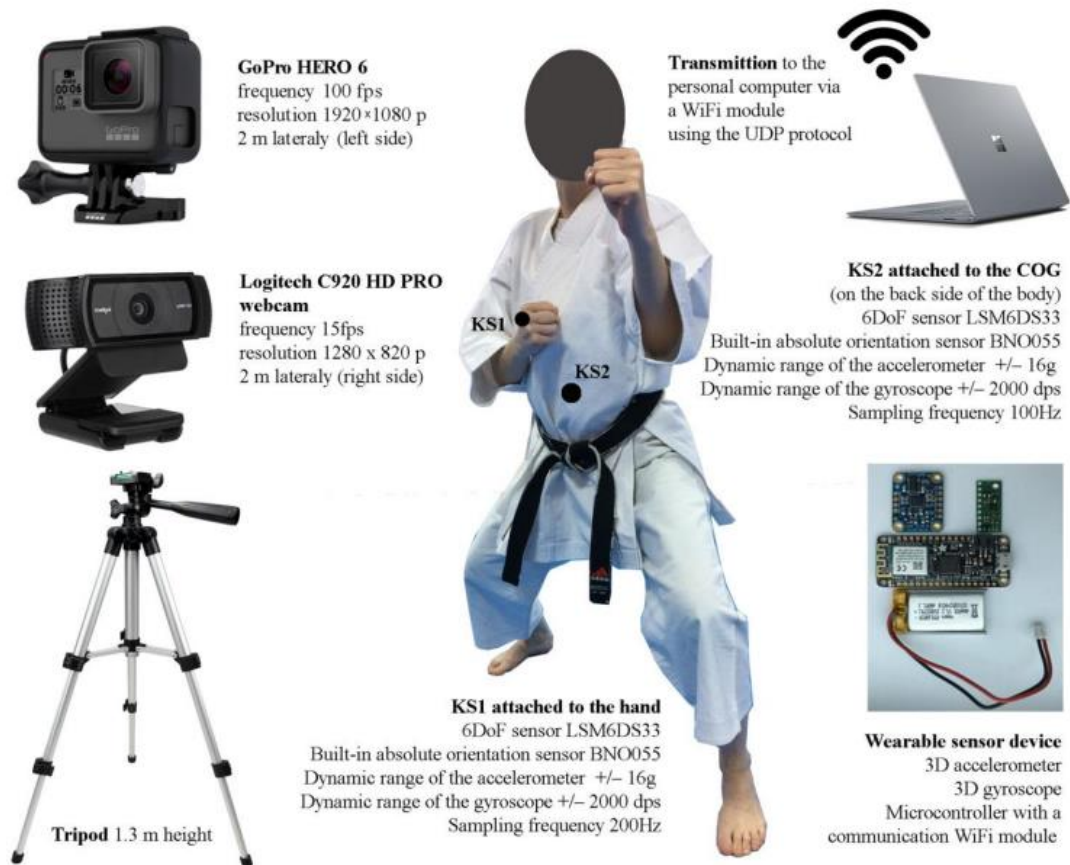
Figure 6.1. The experimental equipment consisted of a pair of cameras and a laptop that were wirelessly linked to two sensors affixed to the athlete
