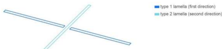
Figure 4. Diagram showing the node with one central lamella and two connecting lamellae when lamellae axes intersect.
